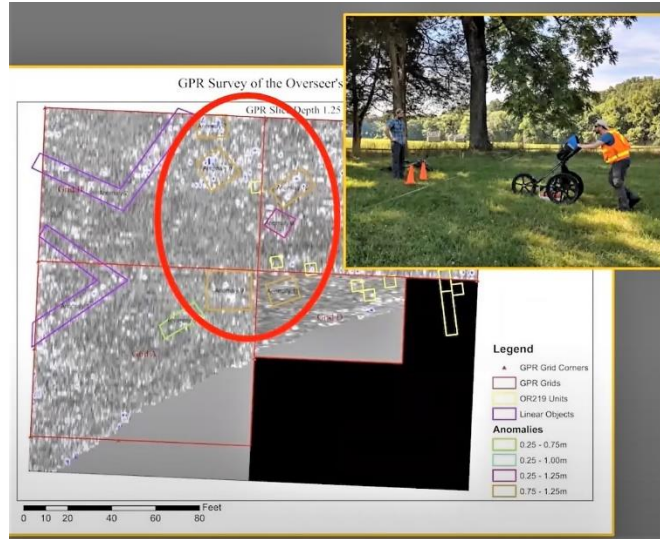
Ground penetrating radar survey of the Overseer's site
