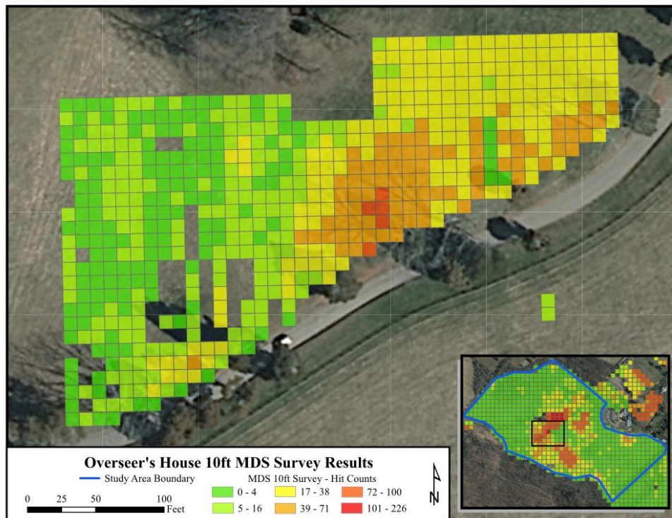
The detailed 10 foot square metal detector survey of the overseer's house site shows numerous detector hits (in the red squares), thus helping to pinpoint the likely location of the structure.
